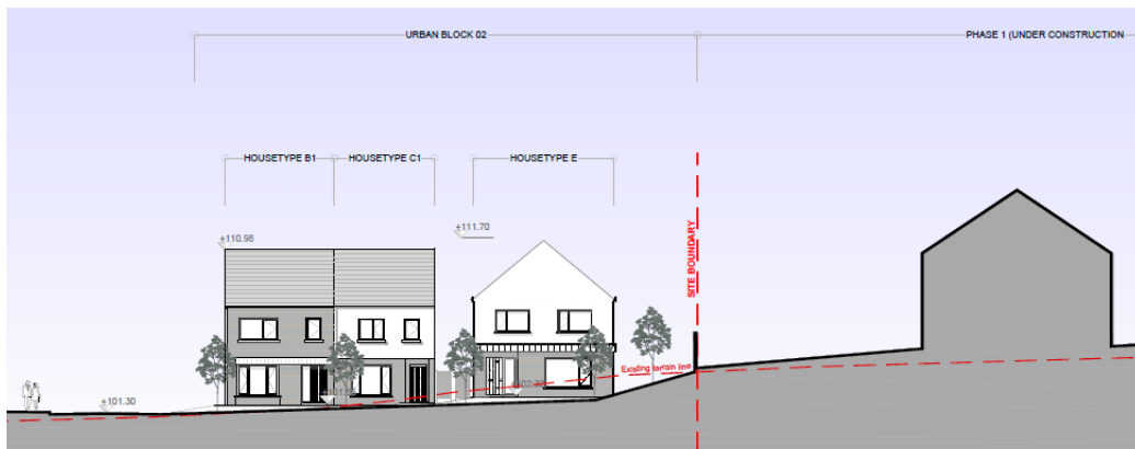
Section 6 Prepared by Reddy Architects Showing relationship between the Proposed Development and Units Under Construction in Phase 1
